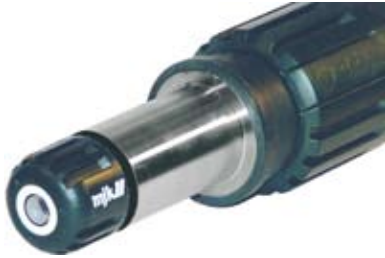
pH electrode, item no. 160310, 1 - 14 pH, 10 - 80 °C, 0 = 4.6 pH.
