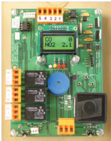
Plug-in connectors and easy access sensors for fast maintenance.
